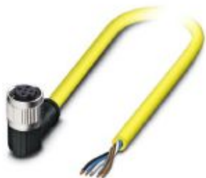
Sensor/actuator cable, 5-position, PVC, yellow, free cable end, on Socket angled M12, coding: A, cable length: 15 m
