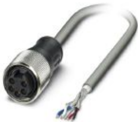
Bus system cable, DeviceNet™, 5-position, PUR halogen-free, silver-gray RAL 7001, shielded, free cable end, on Socket straight 7/8"-16UNF, cable length: 2 m
