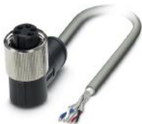
Bus system cable, DeviceNet™, 5-position, PUR halogen-free, silver-gray RAL 7001, shielded, free cable end, on Socket angled 7/8"-16UNF, cable length: 15 m
