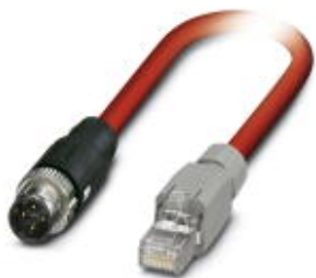
Assembled Sercos III cable, shielded, star quad, 22 AWG stranded (7-wire), RAL 3020 (traffic red), M12 plug, SPEEDCON, 4-pos. to RJ45 plug/IP20, length: 7.5 m
