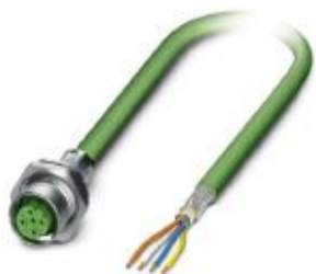
Assembled EtherCAT ® cable, shielded, star quad, AWG 22 stranded (7-wire), RAL 6018 (yellow-green), M12 flush-type socket, 4-pos. on free conductor end, length: 1 m
