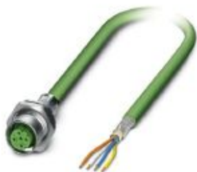
Assembled EtherCAT ® cable, shielded, star quad, AWG 22 stranded (7-wire), RAL 6018 (yellow-green), M12 flush-type socket, 4-pos. on free conductor end, length: 2 m
