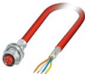
Assembled Sercos III cable, shielded, star quad, AWG 22 stranded (7-wire), RAL 3020 (traffic red), M12 flush-type socket, rear mounting, SPEEDCON 4-pos. on free conductor end, length: 0.5 m
