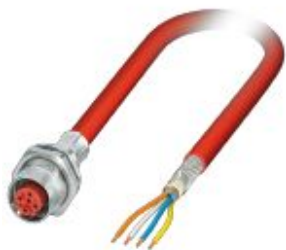
Assembled Sercos III cable, shielded, star quad, AWG 22 stranded (7-wire), RAL 3020 (traffic red), M12 flush-type socket, rear mounting, SPEEDCON 4-pos. on free conductor end, length: 5 m
