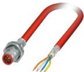
Assembled Sercos III cable, shielded, star quad, AWG 22 stranded (7-wire), RAL 3020 (traffic red), M12 flush-type plug, rear mounting, SPEEDCON 4-pos. on free conductor end, length: 2 m
