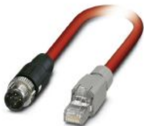
Bus system cable, Sercos CAT5 (100 Mbps), 4-position, PVC, Red RAL 3020, Plug straight M12 SPEEDCON / IP67, coding: D, on Plug straight RJ45 / IP20, cable length: 2 m
