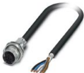
Flush-type socket, shielded, 5-pos., M12, A-coded, rear/screw mounting with M16 thread, with 2 m cable, 5 x 0.34 mm 2
