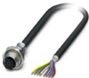
Flush-type socket, shielded, 8-pos., M12, A-coded, rear/screw mounting with M16 thread, with 2 m cable, 8 x 0.25 mm 2
