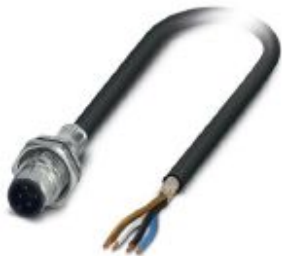
Flush-type plug, shielded, 4-pos., M12, A-coded, rear/screw mounting with M16 thread, with 2 m cable, 4 x 0.34 mm 2
