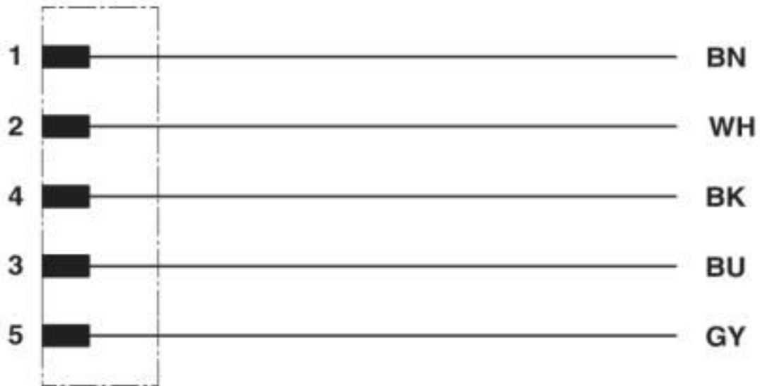
Contact assignment of the M12 plugs
