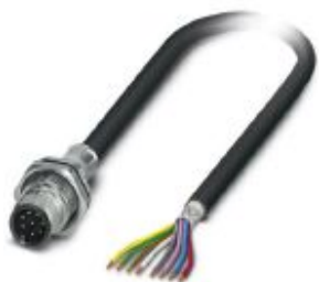
Flush-type plug, shielded, 8-pos., M12, A-coded, rear/screw mounting with M16 thread, with 1 m cable, 8 x 0.25 mm 2
