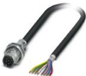
Flush-type plug, shielded, 8-pos., M12, A-coded, rear/screw mounting with M16 thread, with 2 m cable, 8 x 0.25 mm 2
