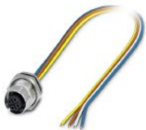
Flush-type connector, 4-position, Socket, straight, M12, D-coded, Rear mounting, M16 x 1.5, Individual wires, cable length: 0.5 m, 0.34 mm 2 , TPE litz wire
