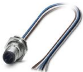
Sensor/actuator flush-type plug, 5-pos., M12 SPEEDCON, A-coded, rear/screw mounting with M16 thread, with 0.5 m TPE litz wire, 5 x 0.34 mm 2
