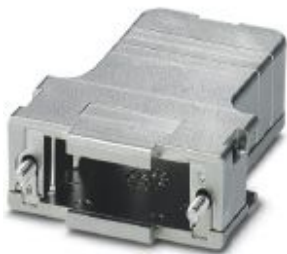
D-SUB sleeve housings, degree of protection: IP20, material: ABS, metal-plated, cable outlet: angled, size of housing: 2, color: Bare metallic
