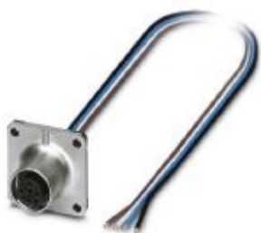
Sensor/Actuator flush-type socket, 4-pos., M12, A-coded, front/square flange mounting, with 0.5 m TPE litz wire, 4 x 0.34 mm 2
