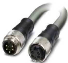
Power cable, 5-position, PUR, gray RAL 7001, Plug straight 7/8"-16UNF, coding: A, on Socket straight 7/8"-16UNF, coding: A, cable length: 0.3 m, 2.5 mm 2 conductor cross section, For power supply
