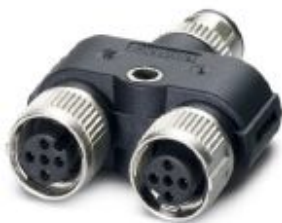
Y distributor, 5-position, shielded, Plug straight M12 SPEEDCON, coding: A, on Socket straight M12 SPEEDCON, coding: A and Socket straight M12 SPEEDCON, coding: A, Parallel distributor
