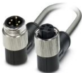
Bus system cable, DeviceNet™, 5-position, PUR halogen-free, silver-gray RAL 7001, shielded, Plug angled 7/8"-16UNF, on Socket angled 7/8"-16UNF, cable length: 15 m
