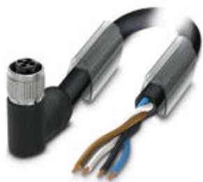
Power cable, 4-position, PUR halogen-free, black-gray RAL 7021, Socket angled M12, on free cable end, cable length: 20 m
