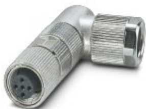
Connector, Universal, 5-position, shielded, Socket angled M12, Coding: A, Crimp connection, knurl material: Zinc die-cast, nickel-plated, external cable diameter 4.5 mm ... 7.5 mm, without crimp contacts
