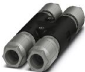
H distributor, QUICKON connection, number of positions: 4, 1 mm 2 ... 2.5 mm 2 , 690 V, 20 A, gray, with four QUICKON nuts, cable diameter range: 6 mm ... 10 mm
