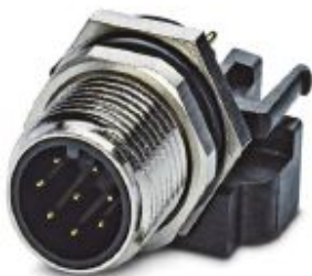
Sensor/actuator flush-type plug, 8-pos., M12, A-coded, rear/screw mounting with M12 thread, with polarity protection, with straight solder connection
