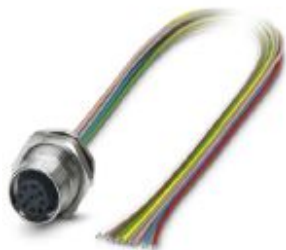
Sensor/actuator flush-type socket, 8-pos., M12 SPEEDCON, rear/screw mounting with Pg9 thread, with 2.0 m TPE litz wire, 8 x 0.25 mm 2
