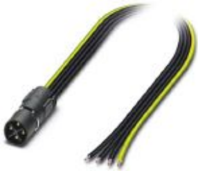
Assembled contact carrier and insulating body, S-coding, 3-pos. + PE, 0.5 m long litz wires
