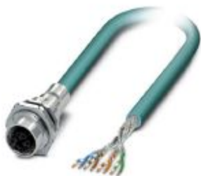
Assembled Ethernet cable, CAT6 A , shielded, 4-pair, 26 AWG stranded (7-wire), RAL 5021 (water blue), M12 flush-type socket, rear/screw mounting with M16 thread to free cable end, length: 0.5 m
