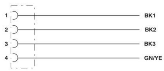
Contact assignment of the M12 socket
