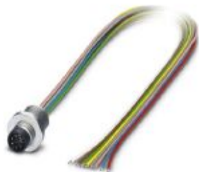
Flush-type connector, 8-position, Plug, straight, M8, Front mounting, M10, Individual wires, cable length: 0.5 m, 0.14 mm 2 , PVC litz wire
