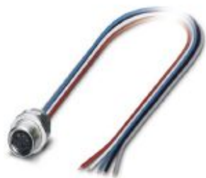
Flush-type connector, DeviceNet™, 5-position, Socket, straight, M8, Front mounting, M10, Individual wires, cable length: 0.5 m, 0.25 mm², PVC litz wire
