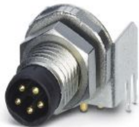
Sensor/actuator flush-type connector, plug, 5-pos., DeviceNet, M8, rear/screw mounting with M10 fastening thread, with angled solder connection
