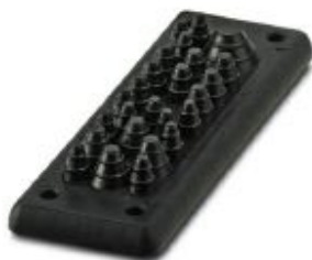
Cable feed-through plates, no. of conductors: 25, length: 154 mm, width: 56 mm, height: 20 mm, external cable diameter: 3x 3 mm ... 6 mm , color: black
