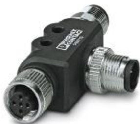
T distributor, PROFIBUS DP (12 Mbps), 5-position, shielded, Socket straight M12, coding: B, on Plug straight M12, coding: B and Plug straight M12, coding: B, Thread M12 plug input not rotatable
