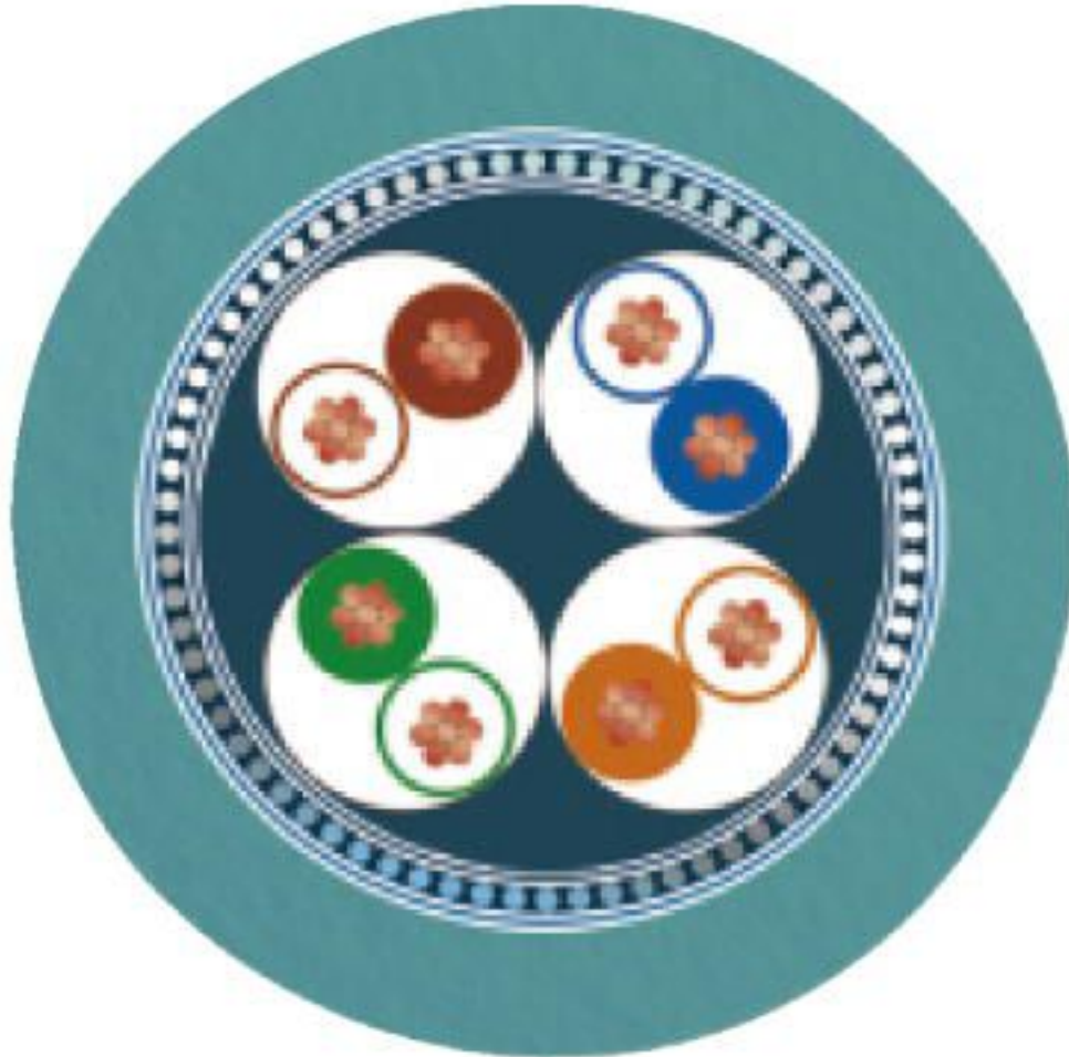
Cable cross section
