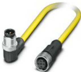
Sensor/actuator cable, 5-position, PVC, yellow, Plug angled M12, coding: A, on Socket straight M12, coding: A, cable length: 0.5 m
