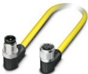
Sensor/actuator cable, 5-position, PVC, yellow, Plug angled M12, coding: A, on Socket angled M12, coding: A, cable length: 0.5 m
