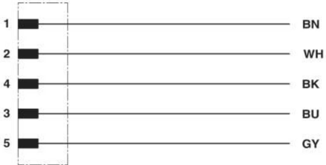
Contact assignment of the M12 plug
