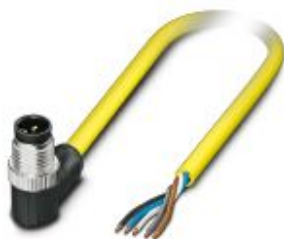
Sensor/actuator cable, 5-position, PVC, yellow, Plug angled M12, coding: A, on free cable end, cable length: 10 m
