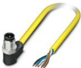
Sensor/actuator cable, 5-position, PVC, yellow, Plug angled M12, coding: A, on free cable end, cable length: 2 m
