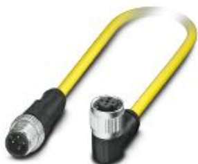
Sensor/actuator cable, 4-position, PVC, yellow, Plug straight M12, coding: A, on Socket angled M12, coding: A, cable length: 0.5 m
