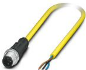
Sensor/actuator cable, 3-position, PVC, yellow, Plug straight M12, coding: A, on free cable end, cable length: 2 m
