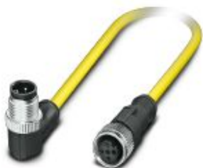
Sensor/actuator cable, 3-position, PVC, yellow, Plug angled M12, coding: A, on Socket straight M12, coding: A, cable length: 1.5 m
