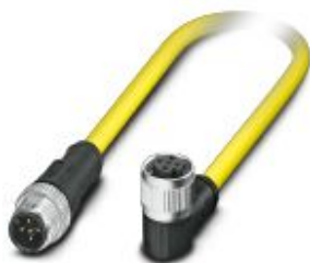
Sensor/actuator cable, 5-position, PVC, yellow, Plug straight M12, coding: A, on Socket angled M12, coding: A, cable length: 1.5 m
