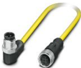
Sensor/actuator cable, 4-position, PVC, yellow, Plug angled M12, coding: A, on Socket straight M12, coding: A, cable length: 3 m
