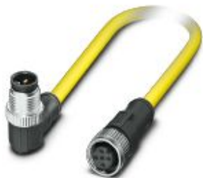
Sensor/actuator cable, 5-position, PVC, yellow, Plug angled M12, coding: A, on Socket straight M12, coding: A, cable length: 5 m
