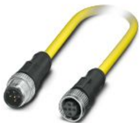
Sensor/actuator cable, 5-position, PVC, yellow, Plug straight M12, coding: A, on Socket straight M12, coding: A, cable length: 3 m
