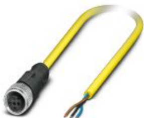
Sensor/actuator cable, 3-position, PVC, yellow, free cable end, on Socket straight M12, coding: A, cable length: 20 m
