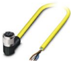
Sensor/actuator cable, 4-position, PVC, yellow, free cable end, on Socket angled M12, coding: A, cable length: 15 m
